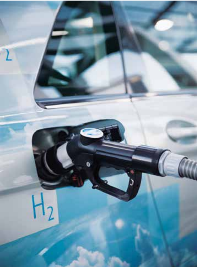
A special dispenser fills the vehicle with the hydrogen
